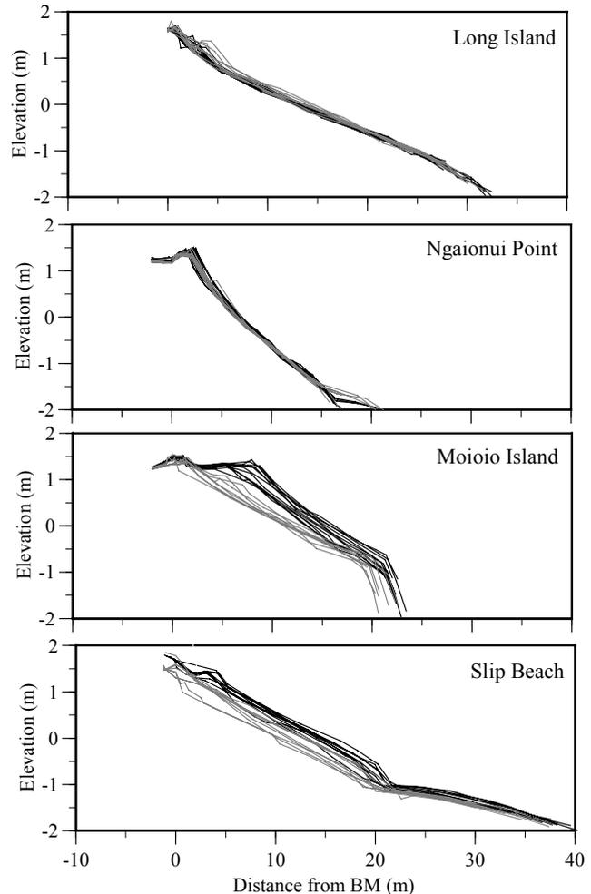
Figure 4. Beach profiles from 4 of the 21 study sites. Lines plotted in grey are from prior to December 2000, after which time HSC were slowed to 18 knots.
