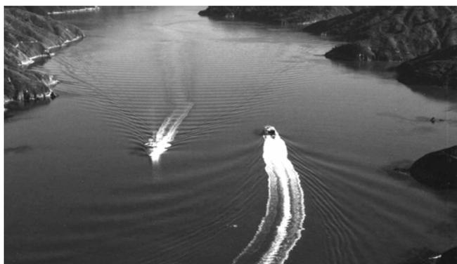
Figure 1. A conventional ship with  $F_{nh} < 1$  (left) and a HSC with  $F_{nh} > 1$  (right) in Tory Channel (Photograph: Marlborough District Council; photographer Graeme Matthews)
