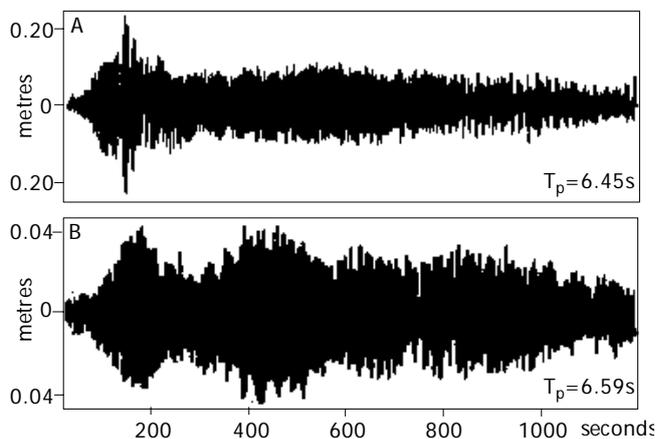
Figure 7. (A) Conventional vessel wake (Aratere, travelling towards Picton), measured in deep water near the sailing line (Figure 6); (B) the same wake measured at site Lissaman's Bay (Figure 6), commencing 19m21s after the start of the wake at the site near the sailing line.
