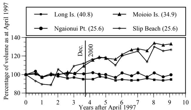
Figure 5. Beach volumes for selected profiles, expressed as a percentage of the volume at April 1997. Numbers in brackets are the initial volumes (m<sup>3</sup>/m).
